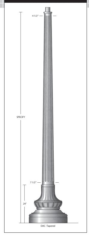
CONSTRUCTION - Durable corrosion resistant cast aluminum base with hand hole and cover. The pole is made of heavy-wall fluted, tapered cast aluminum.
